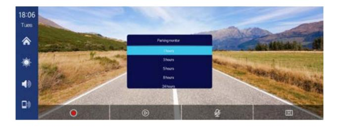
When it prompts "whether to enter the parking monitoring, please pay attention to the battery power", the 5S does not operate, and the system automatically Automatic access to 3-hour parking monitoring
